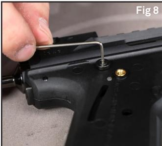
2 Once grips are removed, using a  $\frac{1}{16}$ " hex wrench remove the right side safety lever. (Fig 7)
